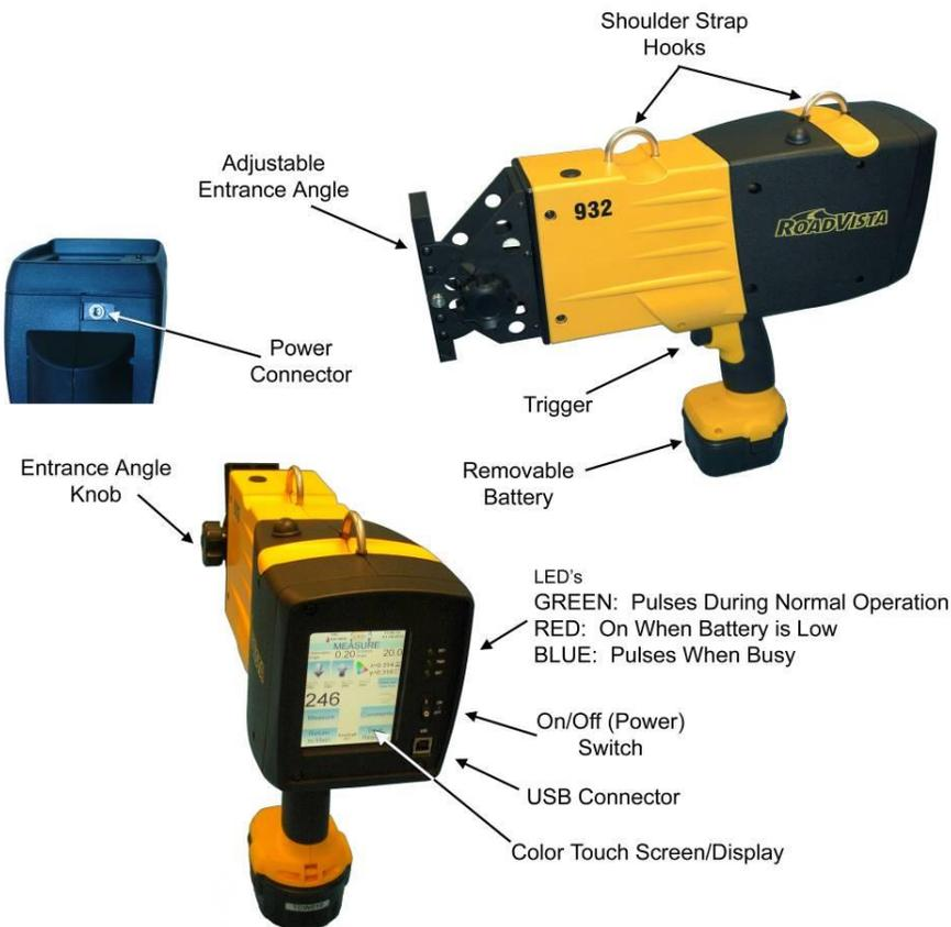
**Figure 2.2-1 Model 932 Mechanical Features**
