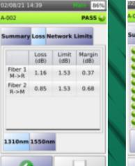
As part of the four second Autotest, TestPro will perform the following measurements for both Singlemode and Multimode.
