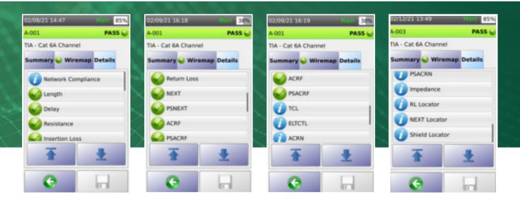
TestPro supports testing and certification for network deployments up to 40 Gigabit Ethernet for Cat 5e, 6, 6A, 7, 8 or Class I/II cabling system. The electrically centered test plug assures the Level 2G/VI accuracy required to support field testing to Cat 8 / Class I/II, and actually exceeds the 2000 MHz requirement, to offer a 3000 MHz platform. As a result, you can feel confident in results over the full frequency range.
